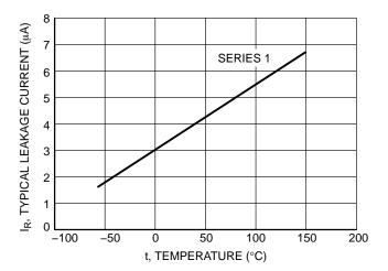
Figure 5. Typical Leakage Current versus Temperature
